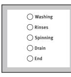
After the machine has started, only the running phase pilot light stays on.
